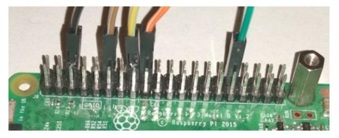
Once you have the wiring setup between the Pi and Cluster Triple ensure all Compute modules have been removed from the Triple, power the Cluster Triple via the "PWR" port, remove any cables from the "USB" port on the Triple, power on the Pi.
