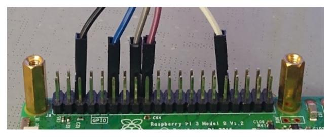
Once you have the wiring setup between the Pi and Cluster Triple ensure either the backplane is disconnected from the ClusterCTRL Controller, power the ClusterCTRL Stack via the barell jack, remove any cables from the "USB" port on the ClusterCTRL Controller and power on the Pi.
